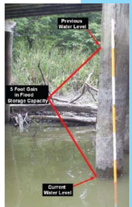
Comparison of water lines before and after flood control efforts by Iberville Parish, which have saved homes from flooding.
